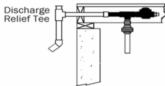
Pump mounted on side of ceiling joist; discharge straight to exterior
