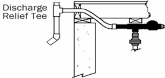
Pump mounted underneath ceiling joist with flexible discharge hose sloped upward and out through exterior wall.
