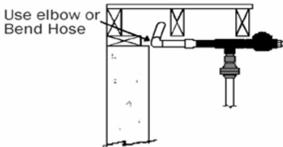
Pump perpendicular to ceiling joist, discharged at right angle from pump through hole to exterior
