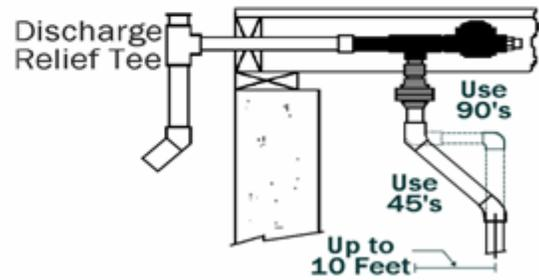
Suction pipe offset using two 45 or 90 degree elbows to clear obstacles or to facilitate installation.
