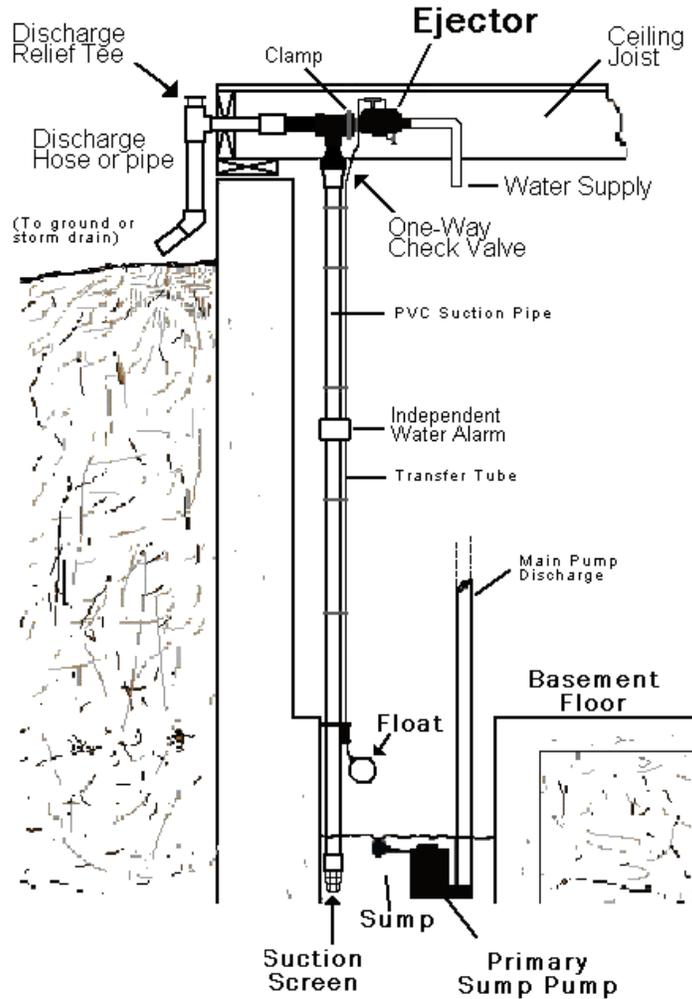
Installing a standard dedicated discharge for your backup pump is the preferred option over installing the backup pump into the same discharge pipe as your primary sump pump. Should your primary sump pump discharge clog, freeze solid, or fail in some other way, your backup pump will still operate correctly when installed on it's own dedicated discharge.
