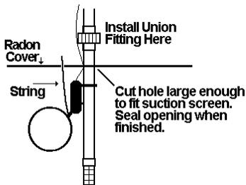
*Preferred Installation* - Your WP-Series pump can be installed in a sump pit with radon seal as shown in the figure at left. In this case the transfer tube should be installed through the same hole as the suction tube and the hole in the radon cover should be sealed with silicone caulk. You may also like to drill a small hole through the cover and feed string to the float to facilitate testing of the pump.
